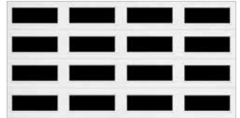
Windows may be arranged vertically or horizontally on Colonial, Ranch and Contemporary designs. Windows placed in the bottom section of a door must use DSB 1/8", or tempered, or 1/2" insulated glass.
